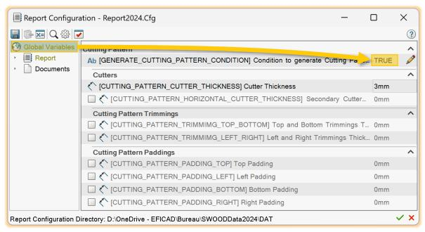
The rest of the parameters in the "Cutting pattern" section can be modified to fine-tune the optimization result, such as saw thickness or cutting margins.
